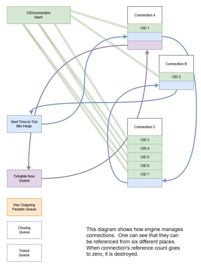
In the diagram above, you can see that the CID-to-connection hash has several links to the same connection. This is
